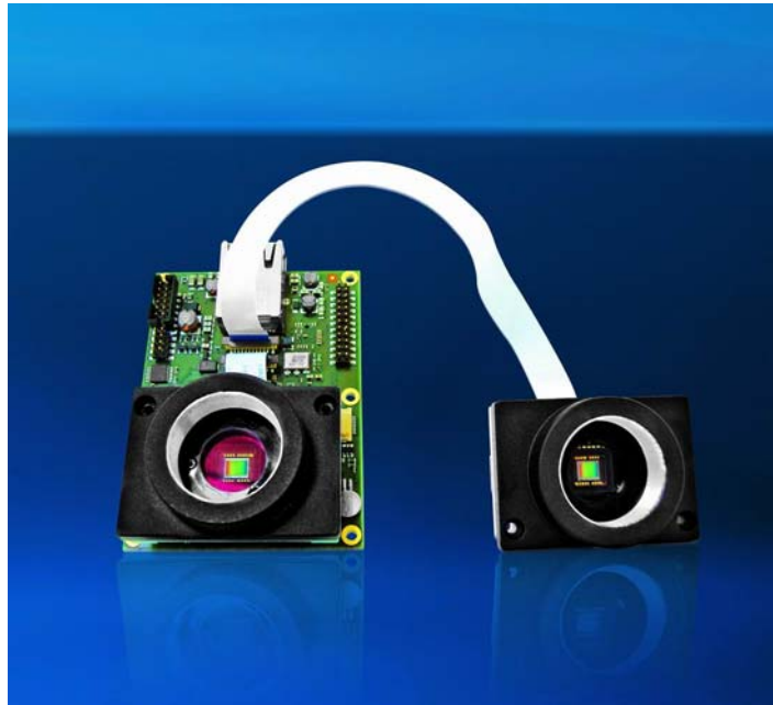
VCSBC64XX Single Board Camera with two mounted sensor boards
