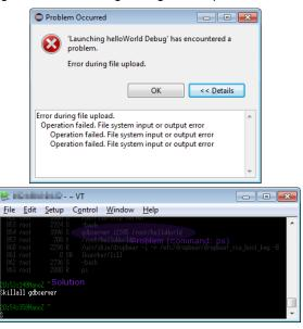
*gdbserver* followed by your binary location. The line starts with a *PID* number, the process ID. Each running program at the camera has such a unique processes ID. You can use the *PID* of your process to terminate it by using the following command: *kill -15 PID*. It sends a request to the gdbserver to quit. In case this does not succeed, you can tell the linux kernel to terminate the process by sending the command *kill -9 PID*.
