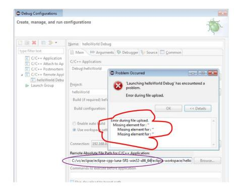
If you get the error message above, it is probably due to a wrong path entered for "Remote absolute file path" in the Debug Configuration window.
