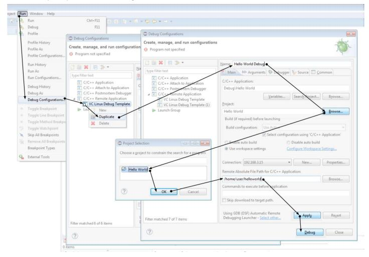
After clicking the Debug button the IDE asks to switch to the so-called Debug Perspective – Accept it.
